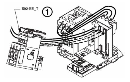
**E1** Plus Overload Relay with Automatic/Manual Reset, Field Selectable Trip Class 10, 15, 20, or 30, Phase Loss Protection Order the replacement overload relay catalog number from the table below. For example, the E1 Plus Class 10 overload relay for a 509-TOD-S1A would be ordered as catalog number 592S-EEPT. If the Overload Panel Adapter needs to be replaced, order part number 193-EPB. The 193-EPB panel adapter is compatible will all of the E1 Plus overload listed in the table below.
